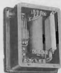
No. 501A Type Desk Set Box Cover Removed
