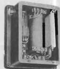
No. 501A Desk Set Box Cover Removed
