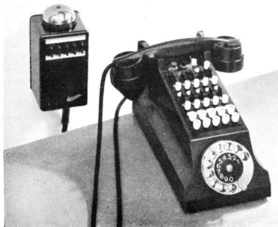
Fig. 6 Operator's set keyboard in front, individual keys and lamps for 10 public exchange lines, at the back common keys and lamps; to left, wall fitting with night switches
