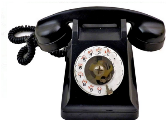
French phone (table and wall model) based on Ericsson's DBH1000 with French dial
