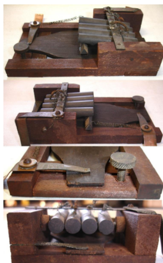
1889 Harrison International Telephone Transmitter US Patent filed 8-9-1889 & issued 5-31-1892
